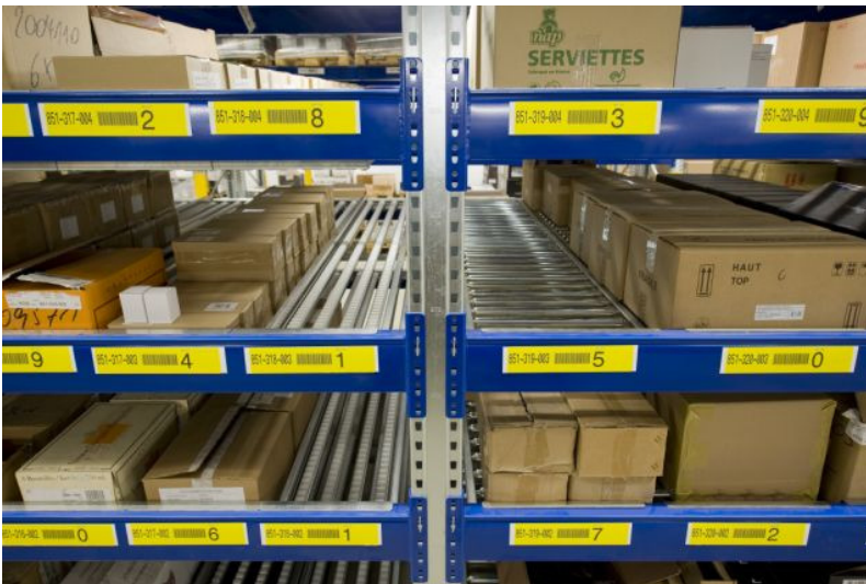
Picture 1: BITO Adapta-Flow modules allow rapid and cost efficient reconfiguration of existing static pallet racking levels into a live storage levels.
